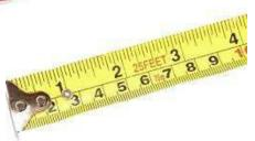
The tape measure should be of a durable quality: retractable, with <u>both metric and imperial markings</u>, a locking clamp, metal case and at least 5m or 20ft long.
