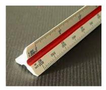
There are many types of scales with various calibrations. The metric scale required to be purchased – which includes 1:20, 1:50 and 1:100 scales - is the most commonly-used scale. (Note that metric scales are proportional and that 1:1, 1:10 and 1:100 scales are really the same – we'll discuss this further in Studio.)
